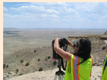
Below: Robotic camera on South Mesa for 360 degree photography
