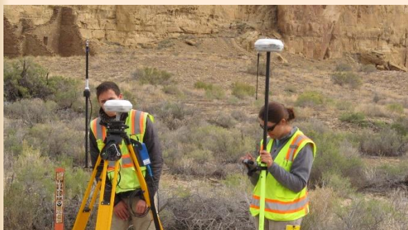
Real Time Kinetic Base Station for subcentimeter control of subsurface Ground Penetrating Radar
